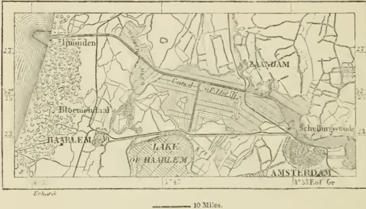
fore, to construct a new canal, the engineers naturally choosing the narrow neck of land known as *Holland op zijn smalst*. This canal of the Y, constructed since 1858, has a length of 25,886 yards, and is 207 feet in width. Its depth, as far as the great flood-gate at Ymuiden, is only 13 feet, but beyond it deepens to 25 feet. The harbour at Ymuiden is formed by two piers, each 5,000 feet in length, and covers an area of 297 acres. The entire work cost nearly
