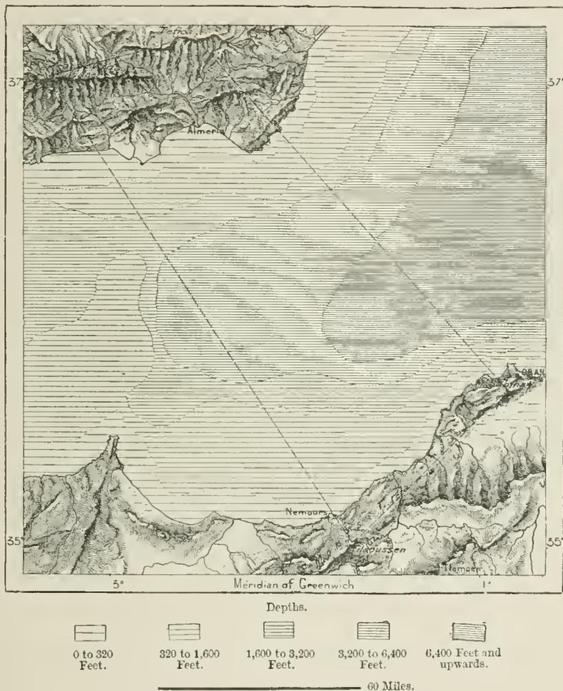
range, and Msabiha in the neighbouring Oran group. The chain of triangles is now continuous from the northernmost islet in Shetland to the 34th parallel of latitude in Algeria, and will soon be extended far into the Sahara, forming the largest arc of the meridian that has hitherto been astronomically measured on the surface of the globe.
