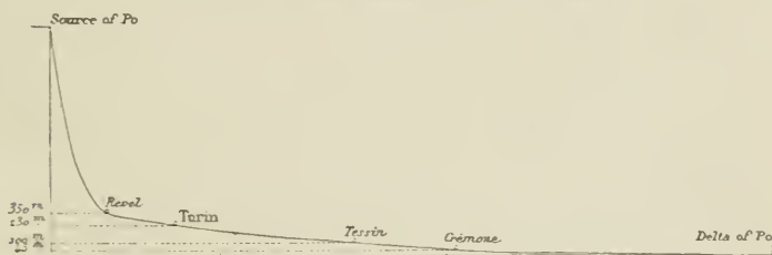
Fig. 54.—SLOPE OF THE VALLEY OF THE PO. The vertical scale is ten times larger than the horizontal.
