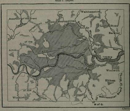
Fig. 90.—The London Sewers. Scale 1: 250,000.
