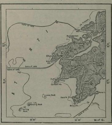
Fig. 231.—Valentia and its Telegraph Cables. Scale 1: 225,000.
