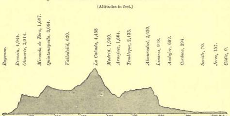
Fig. 139 .- PROFILE OF THE RAILWAY FROM BAYONNE TO CADIZ.
